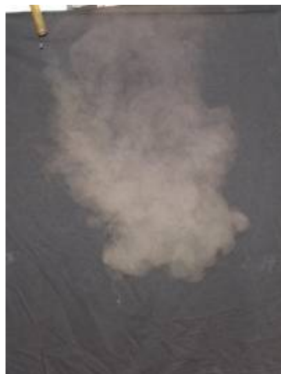
Fig. 1. Photograph of the path of condensed-steam or water droplets projecting downward direction. Photograph shows a stream droplets coming out from a tube downward direction and turning around and move upward. The droplets are visible as a white mist.
